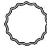
SECTION A-A 16 FLAT FLUTE CROSS SECTION
